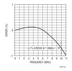
Figure 23. Error Plot for the RMS/DC Converter. Frequency Dependent Gain Boost at A2 Preserves 1% Accuracy, But Causes Slight Peaking Before Roll-Off
