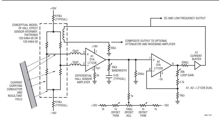
Figure 24. Hall Effect Stabilized Current Transformer (DC  $\rightarrow$  High Frequency Current Probe)
