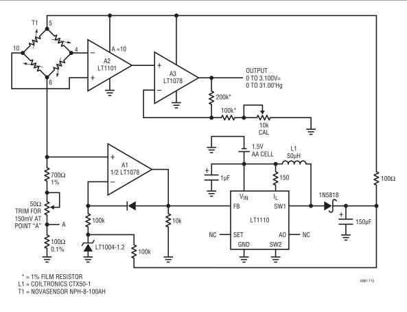
Figure 15. 1.5V Powered Barometric Pressure Signal Conditioner Uses Instrumentation Amplifier and Voltage Boosted Current Loop
