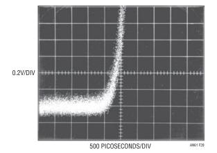
Figure 28. Expanded Scale View of Leading Edge Is Clean with No Trigger Pulse Artifacts. Display Granularity Derives from Sampling Oscilloscope Operation
