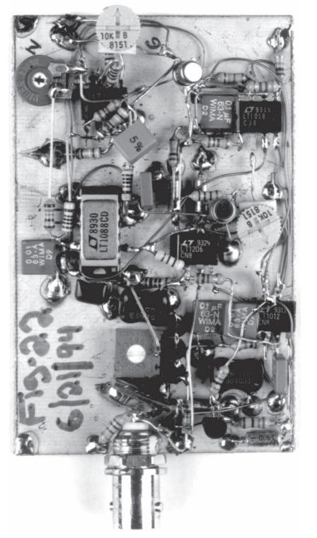
Figure A7. Figure 22's Circuit Puts Entire HP3400 Electronics on One Small Board. FET Buffer-LT1206 Amplifier Appear Left Center Behind BNC Shield. LT1088 IC (Upper Center) Replaces Thermal Converter. LT1013 (Upper Right) Based Circuitry Replaces Photo-Chopper Board. LT1018 and Components (Lower Right) Provide Overload Protection. Ain't Modern ICs Wonderful?
