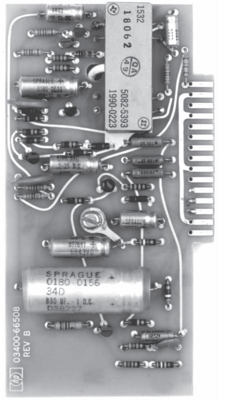
Figure A6. Chopper Amplifier Board Feedback Controlled the Thermal Converter. Over Fifty Components Were Required, Including Neon Lamps, Photocells and Six Transistors. Photo-Chopper Assembly Is at Board's Lower Right
