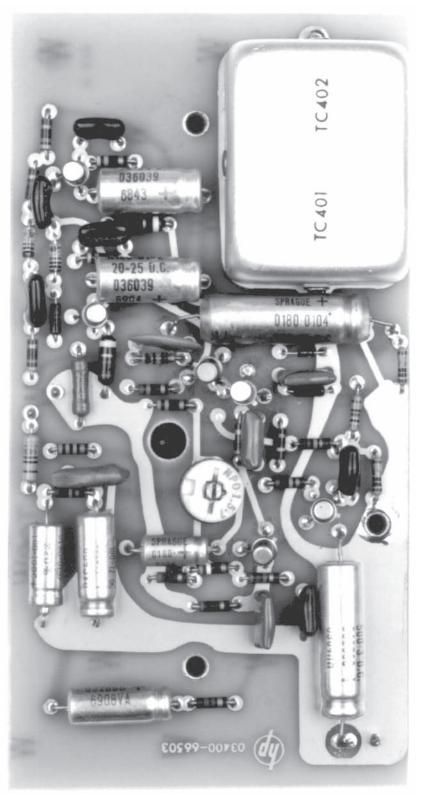
Figure A4. The Voltmeters "Video Amplifier" Received Input at Board's Left Side. Amplifier Output Drove Shrouded Thermal Converter at Lower Right. Note High Frequency Response Trimmer Capacitor at Left Center
