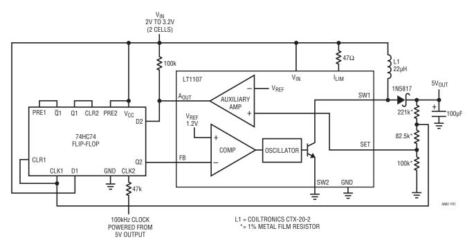
Figure 1. A Synchronizing Flip-Flop Forces Switching Regulator Noise to Be Coherent with the Clock
