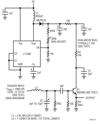
Figure 26. Triggered 250ps Rise Time Pulse Generator. Trigger Pulse Amplitude Controls Output Phase
