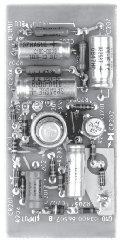
Figure A2. The Hewlett-Packard 34004's Wideband Input Buffer. Nuvistor Triode (Upper Center) Provided Speed, Low Noise, and High Impedance. Circuit Required 75V, –17.5V and –6.3V Supplies. Regulated Filament Supply Stabilized Follower Gain While Minimizing Noise
