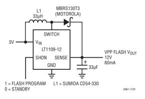
Figure 29. Switching Regulator Provides Complete Flash Memory Programmer
