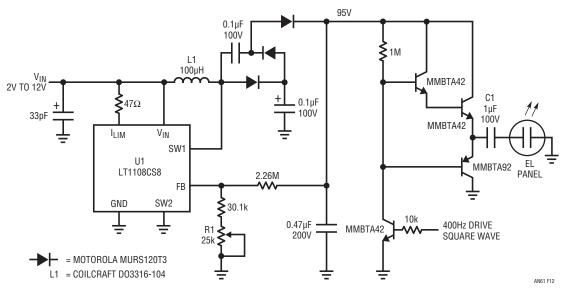
Figure 12. Switch Mode EL Panel Driver Eliminates Large 400Hz Transformer
