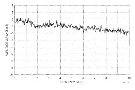
Figure 36. RMS Noise vs Frequency at 5MHz Bandpass Shows Slight Fall-Off Beyond 1MHz
