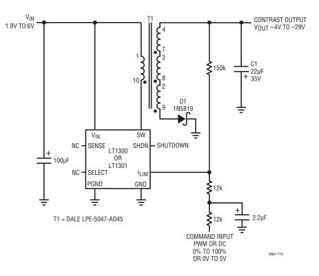
Figure 10. Liquid Crystal Display Contrast Supply Operates from 1.8V to 6V with -4V to -29V Output Range
