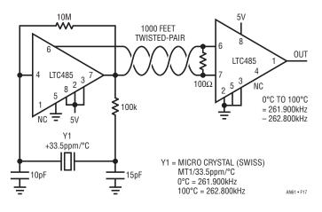
Figure 17. Quartz Crystal Based Circuit Provides Temperature-to-Frequency Conversion. RS485 Transceivers Allow Remote Sensing
