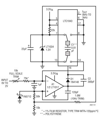
Figure 31. 3.3V Powered Voltage-to-Frequency Converter. Charge Pump Based Feedback Maintains High Linearity and Stability
