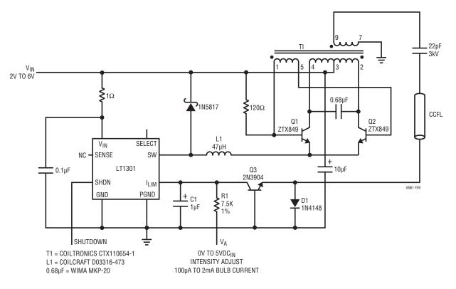
Figure 9. Low Power Cold Cathode Fluorescent Lamp Supply Is Optimized for Low Voltage Inputs and Small Lamps
