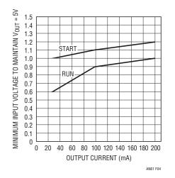
Figure 4. Input-Output Data for the 1.5V to 5V Converter Shows Extremely Wide Start-Up and Running Range into Full Load
