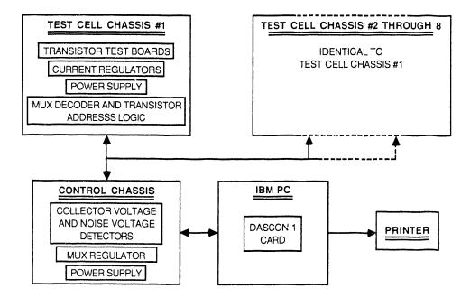
Figure 4. Schematic diagram of the burnin tester.
