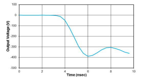
*Figure 5: Series connected pulse generator output terminated into 200Ω RLOAD*
