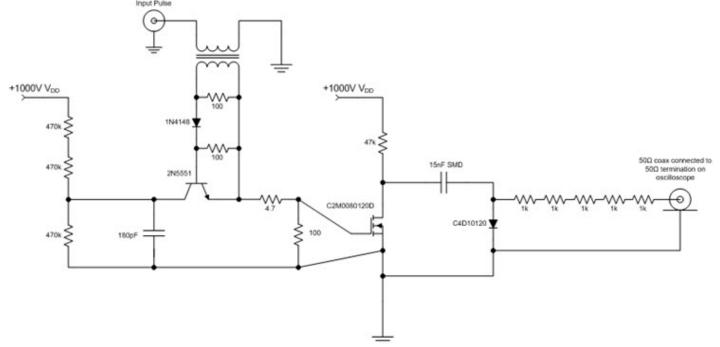
Figure 8: Schematic for the C4D10120A dV/dt ruggedness test setup
