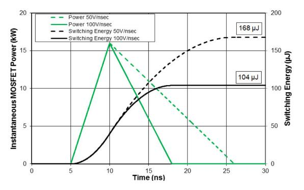
Figure 3: Instantaneous power dissipation and turn-on energy loss for 50V/ns and 100V/ns
