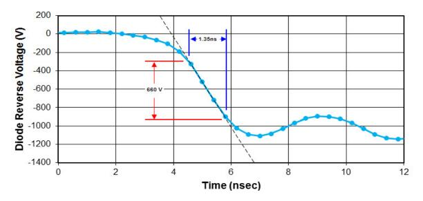
Figure 9: C4D10120A reverse dV/dt = 490 V/ns
