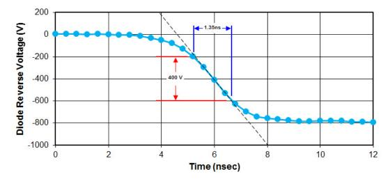
Figure 7: C3D03060A reverse dV/dt = 295 V/ns
