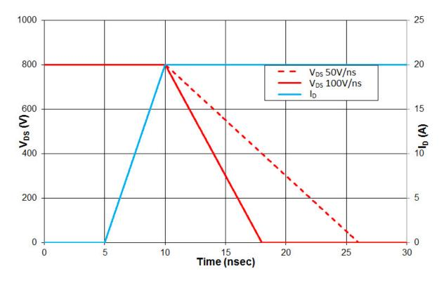
Figure 2: Ideal MOSFET turn-on waveforms for dV/dt limits of 50V/ns and 100V/ns
