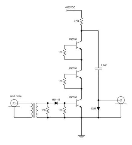
Figure 6: Schematic for the C3D03060A dV/dt ruggedness test setup
